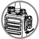
Attach the accessory connector cover when the accessory is not in use.
